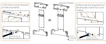
Note: When installing the bracket, be sure to use a spirit level to test and keep the bracket parallel to the horizontal plane
