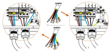
Note: According to the different N terminals of Grid(INV), select the corresponding connection position.(if need:(A + 6.4B) or (I + 6.4II))
